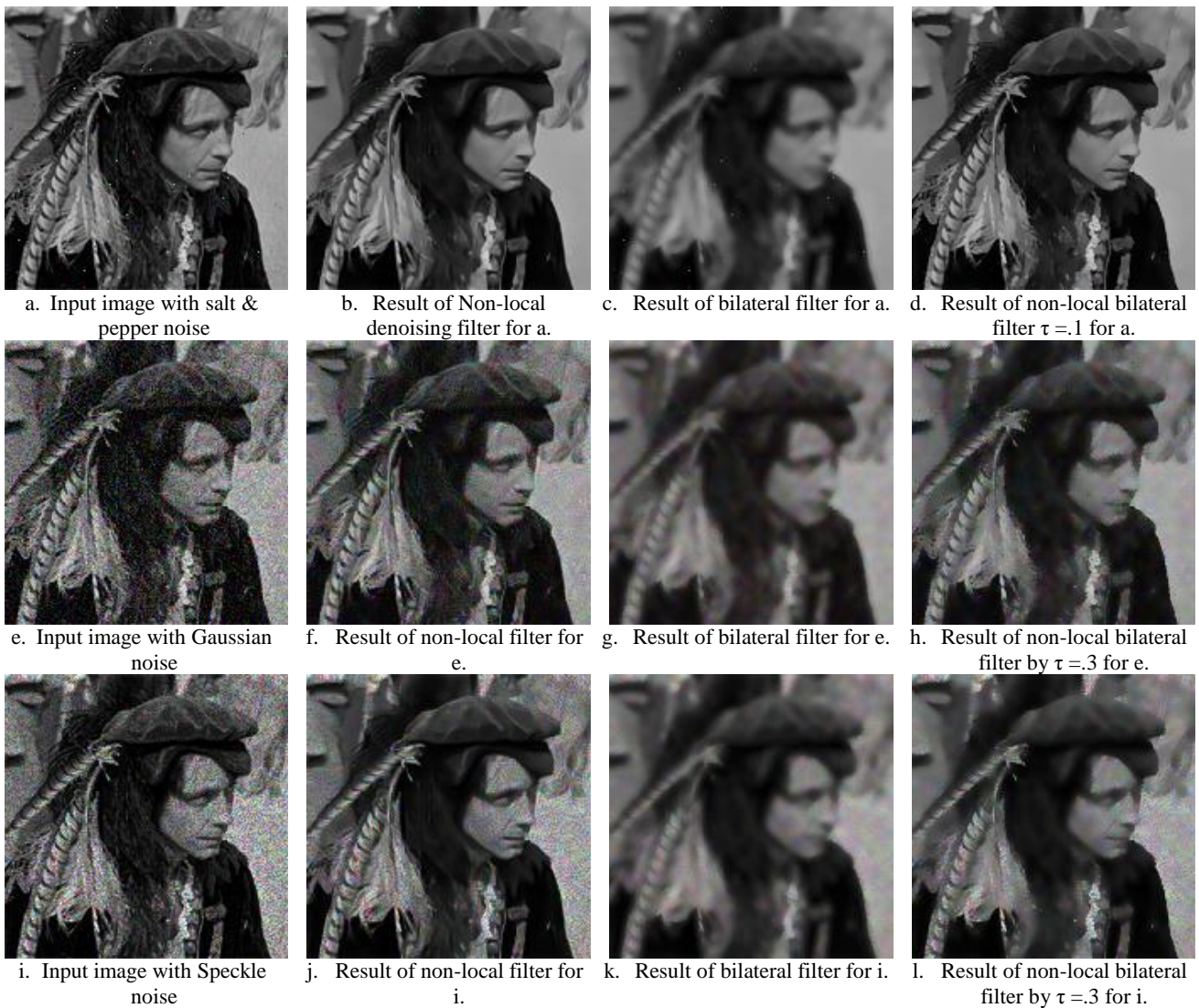
Fig. 2. Effect of Non-local, Bilateral Filter and Non-local Bilateral Filter for gray “man” image
