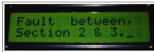
Figure 8 : Fault location displayed on LCD
