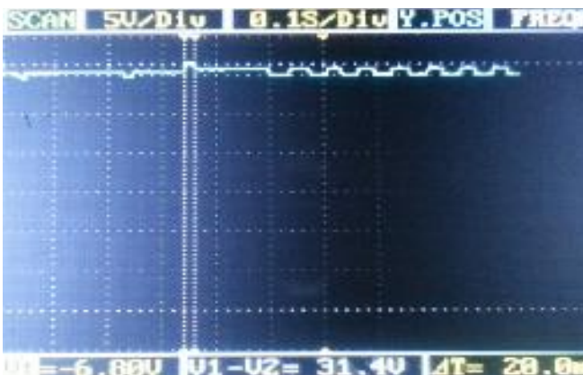
e: R=7.5-15\Omega , V_{in}=24V & V_{ref}=30V (5V/div & 0.1s/div)
