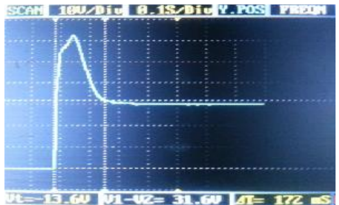
f. R=15\Omega, V_{in}=24V & V_{ref}=30V (10V/div & 0.1s/div)
