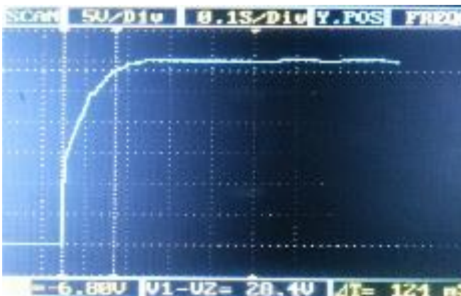
c: R=7.5\Omega , V_{in}=12V & V_{ref}=30V (5V/div & 0.1s/div)
