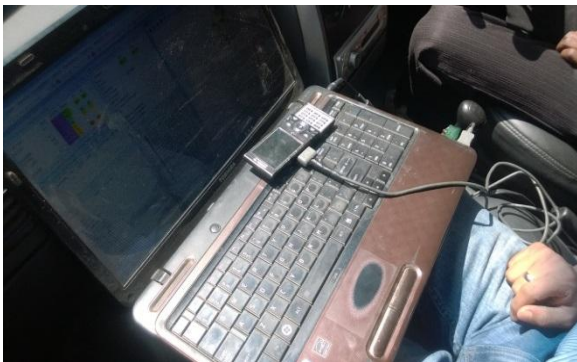
Fig.3 Process of data collection depicted using real-time drive test with TEMS Investigation.
