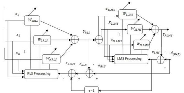
**Fig. 2: Representation of RLMS Algorithm**
