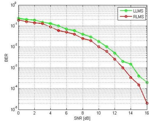
**Fig. 5: BER vs SNR for QPSK MIMO-OFDM system using LLMS and RLMS.**
