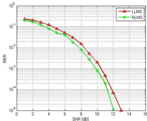
**Fig. 4: BER vs SNR for BPSK MIMO-OFDM system using LLMS and RLMS.**
