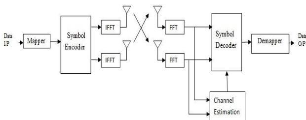
**Fig. 1: MIMO-OFDM system model.**
