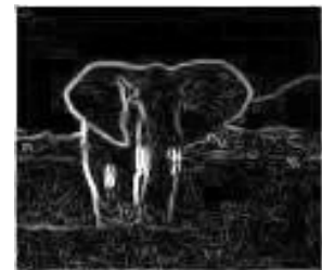
Fig 11. b) Edge detection for original image by Prewitt operator
