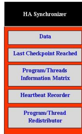
Figure 2. High Availability Synchronizer
