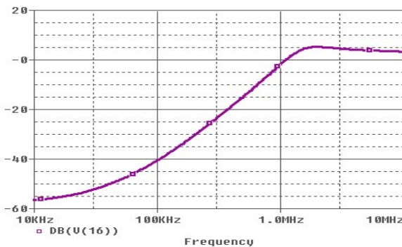
Fig. 8(a): Simulated magnitude response (in dB) for high pass filter with control word [d_2 d_1 d_0 = 0 1 0] selected
