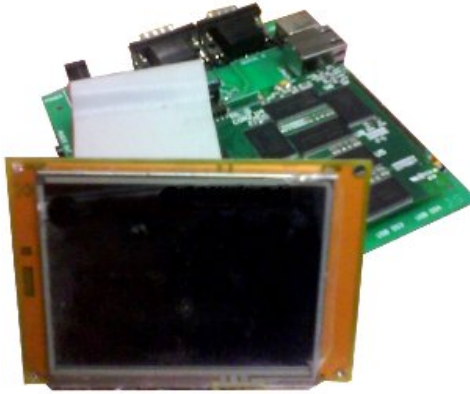
Fig. 2. CID 300/9 industrial motherboard. µC: ARM-920T, CPU: 400 MHz, Ports: 4 USB, 1 Ethernet, 2 Serial, RAM: 128MB, Audio: 2 3.5mm input/output, SD Card: 1 port, Video: Touchscreen and LDVS port, OS: Linux based
