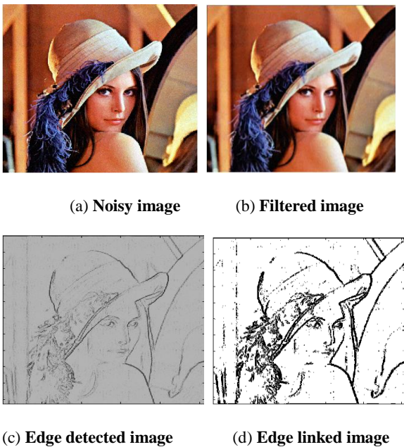
Figure 9: Illustration of fuzzy edge linking algorithm-2 results for Lena image with \sigma = 10
