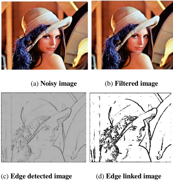
Figure 8: Illustration of fuzzy edge linking algorithm-2 results for Lena image with \sigma = 5
