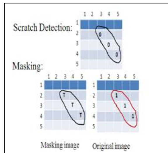
Fig 1: figure demonstrates the scratch detection and masking algorithm. In first matrix 0 value indicate the damaged pixels. In second Boolean matrix, for 0 values in first matrix true value set in Boolean matrix and in third original matrix damaged pixel 's RGB value set to red.
