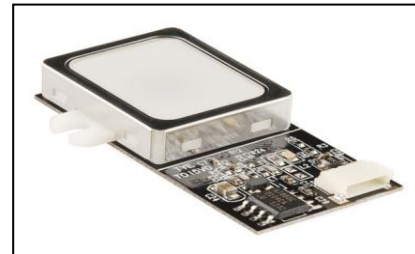
Fig.6. Fingerprint sensor module.
