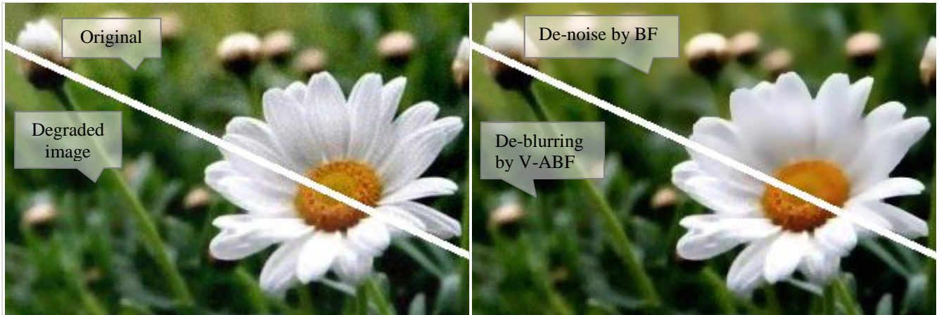
Fig. 1. BF and V-ABF Reduce degree of low resolution and improve major edges. Deblurring example by V-ABF has sharp edges.
