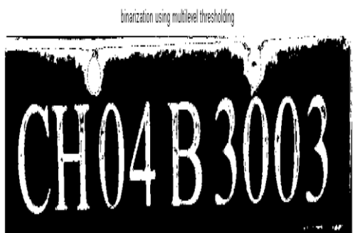
Fig 9: Binarisation using OTSU method with recognition rate of 96.64%
