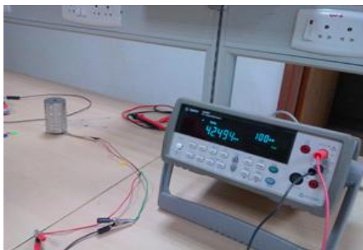
Fig 7: Agilent Multimeter Used For Sensor Calibration
