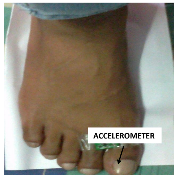
Figure 5: Accelerometer mounted on leg
