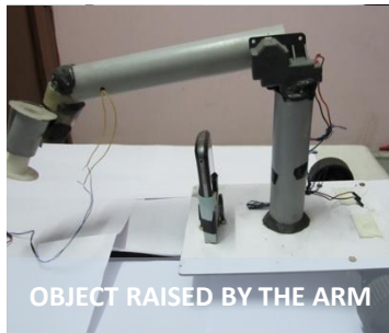
Figure 2: Arm and Gripper in action
