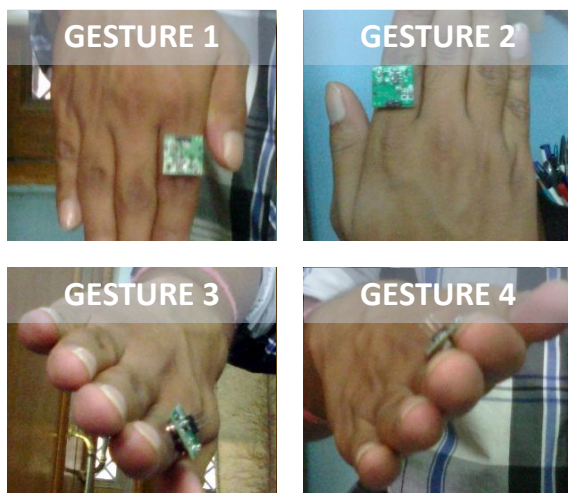
Figure 4: Different hand gestures to control the Robotic Arm (Arm & Gripper) Movement
