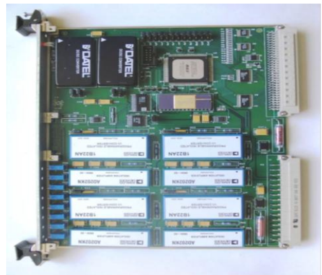
Fig8: VME bus based analog output card
