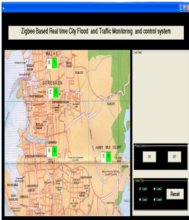
Fig. 6 VB Based Control Panel
