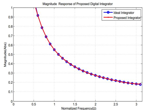
Fig 3: Frequency response of proposed integrator for sampling frequency normalized to  $\pi$  radian
