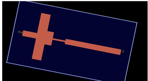
Fig 8: Agilent EMPro layout of first order integrator
