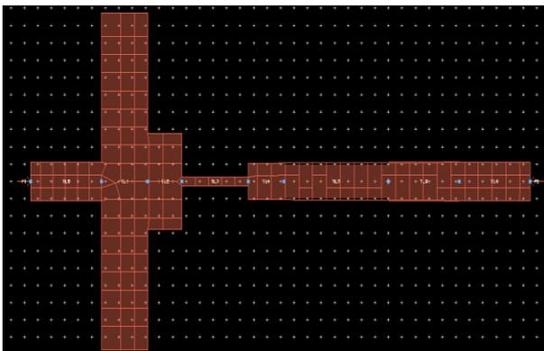
Fig 7: Layout diagram of proposed integrator with six sections of microstrip line
