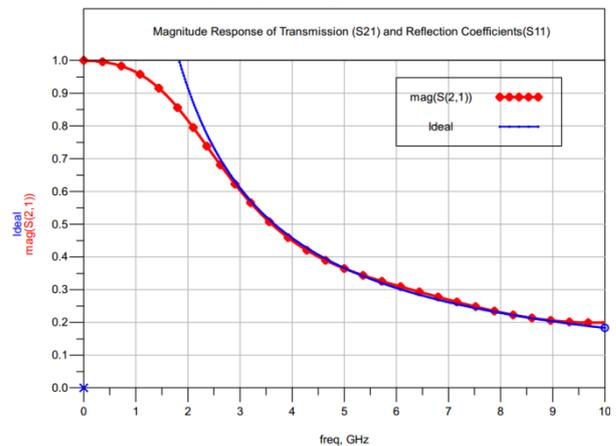
Fig 8: Frequency Response of the proposed 1<sup>st</sup> order integrator and ideal integrator
