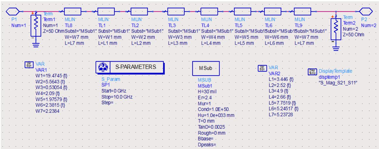
Fig 5: Agilent ADS Schematic of six element transmission line 1st Order Integrator
