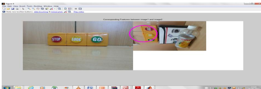
Figure 10. The box is detected in the input image even after different scaling using SIFT
