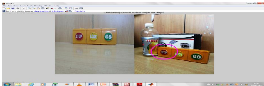
Figure 9. The box is detected in the input image even after different illumination, orientation using SIFT (IMAGE 1)
