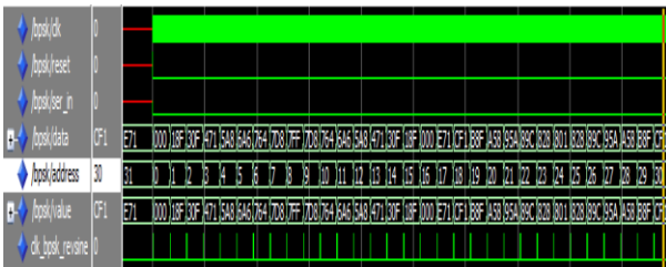
Figure 16: Q-Channel BPSK Signal for 32 address bits
