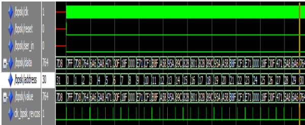
Figure 14: I-Channel BPSK Signal for 32 address bits
