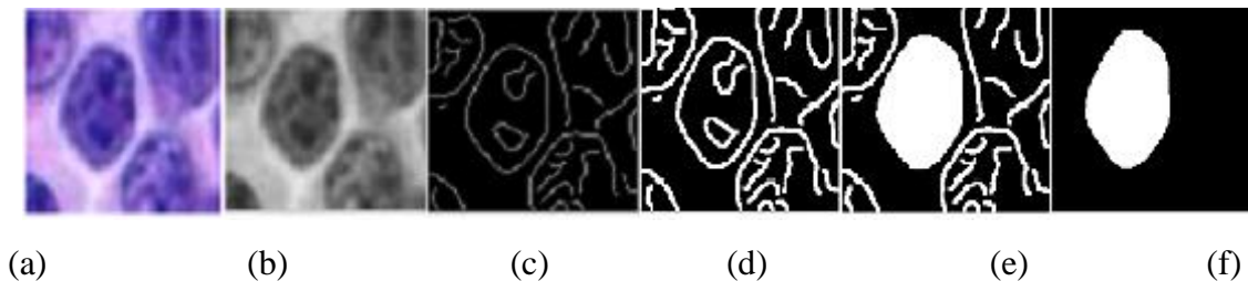
Fig 5. (a) Original image (b) gray image (c) canny edge detection (d) image dilation (e) connected component hole filling of cells (f) max area identification
