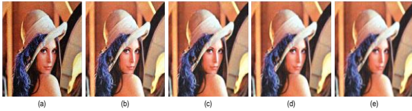
Figure15:Illustration of Absolute distance results for Lena image with \sigma = 20 (a) Noisy image (b) Corresponding output image for (3x3, 3x3) window (c) Corresponding output image for (3x3, 5x5) window (d) Corresponding output image for (3x3, 7x7) window (e) Corresponding output image for (3x3, 9x9) window.
