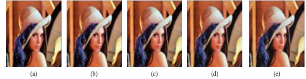
Figure11: Illustration of Minkowski's distance results for Lena image with \sigma=40 (a) Noisy image (b) Corresponding output image for (3x3, 3x3) window (c) Corresponding output image for (3x3, 5x5) window (d) Corresponding output image for (3x3, 7x7) window (e) Corresponding output image for (3x3, 9x9) window
