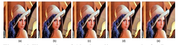
Figure12: Illustration of Absolute distance results for Lena image with \sigma=5 (a) Noisy image (b) Corresponding output image for (3x3, 3x3) window (c) Corresponding output image for (3x3, 5x5) window (d) Corresponding output image for (3x3, 7x7) window (e) Corresponding output image for (3x3, 9x9) window.
