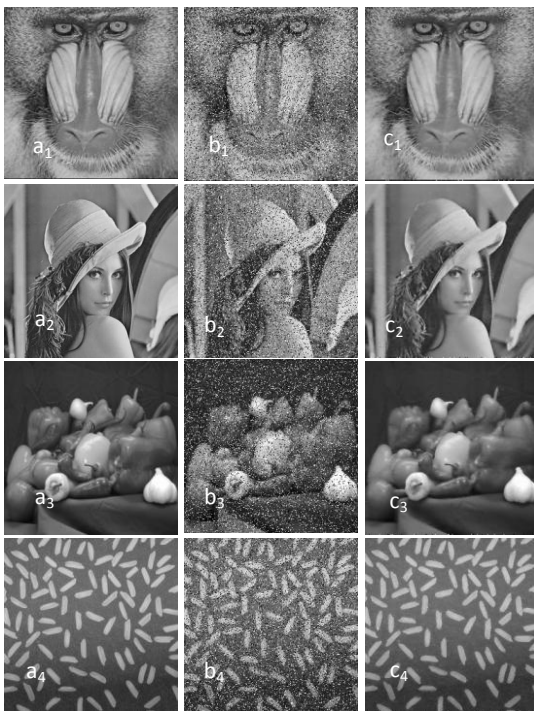
Fig.6 Performance of test images: (a 1,2 and a 4 ) original images,(b 1,2 and b 4 ) images corrupted with 10% of impulse noise and gaussian noise with \sigma=200 and (c 1, 2 and c 4 ) images enhanced by proposed filter
