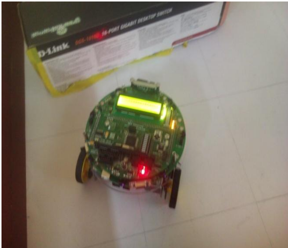
Fig 6: Mobile robot(FIREBIRD kit) follows path planning according to Monte Carlo Localization.
