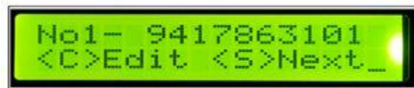
Figure9: Editing/saving numbers on LCD from which SMS is received by GSM module
