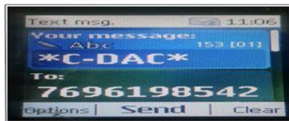
Figure10: SMS (*C-DAC*) send to SIM present in GSM module by the stored number
