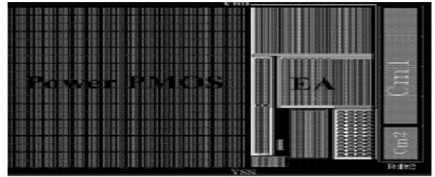
Fig. 9. Layout of the proposed full on-chip CMOS LDO
