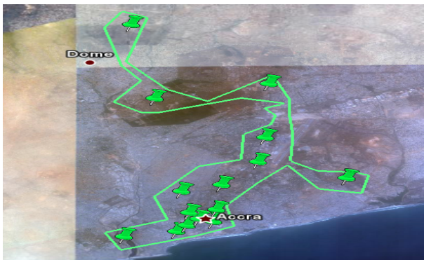
Fig. 8. Initial distributions of WiMAX sites based on coverage simulation
