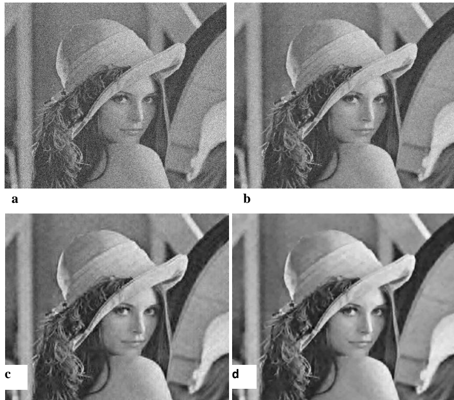
Fig 4: (a) Lena noisy image with \sigma = 25 ; (b) denoised image with TV regularization algorithm, PSNR=26.63; (c) denoised image with PCA in wavelet domain, PSNR=29.26; (d) denoised image with proposed algorithm, PSNR=29.83.
