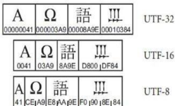
Figure 2: Unicode encoding forms
