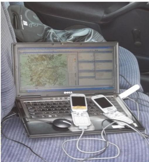
Figure 2: TEMS Measurement Tool used for Field gathering of RSS Data
