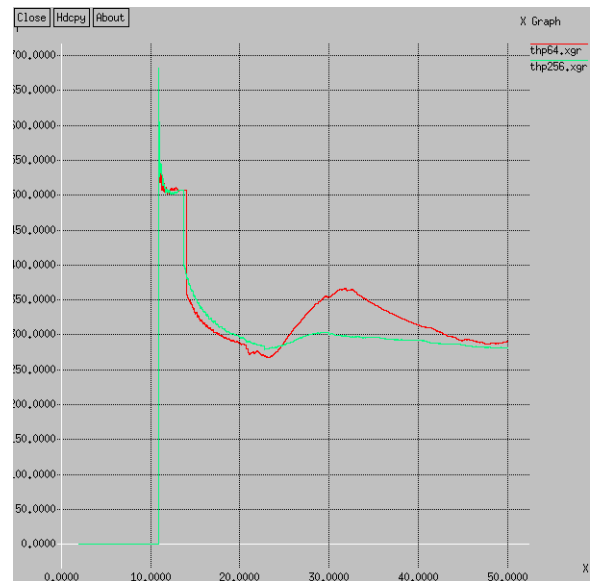
Fig 4.3 . comparision throughput of data moving in SBPN of average packet size 256 kb and 64 kb while doing video confrencing.
