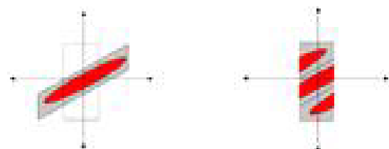
Fig 2: Support of wedge before (left) wrapping and after wrapping
