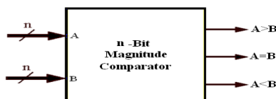
Fig 1: Block Diagram of n-Bit Magnitude Comparator
