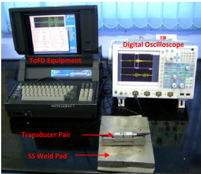
Fig 5: ToFD signal acquisition experimental set-up
