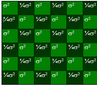
Fig 2: When demosaicing is performed with linear interpolation, the original green pixels have higher variance than the interpolated green pixels. The spatial pattern of variances is the basis for detecting the presence of demosaicing. The green photosites pixel values in the Bayer array are IID with variance \sigma^2 , the above image shows the variance from which each pixel value is drawn.
