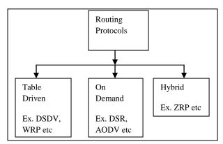
Fig 2: Classification of Routing Protocols for MANETs
