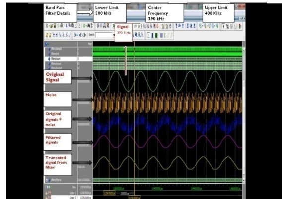
Figure 11. Original signal, noise + signal and filtered signals
