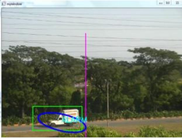
Fig 9: Vertical Trip wire. Alarm for Motion travelling from Rhs toward Lhs side
