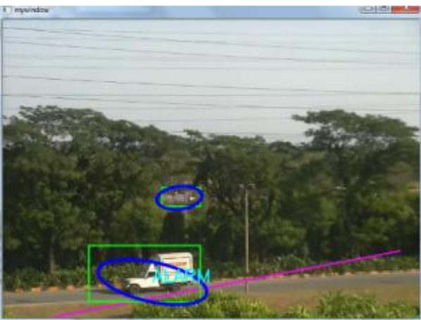
Fig 11: Horizontal Trip Wire. Alarm for Motions travelling from Rhs toward Lhs
