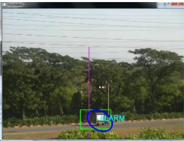
Fig 10: Vertical Trip wire. Alarm for Motion travelling from Lhs toward Rhs
