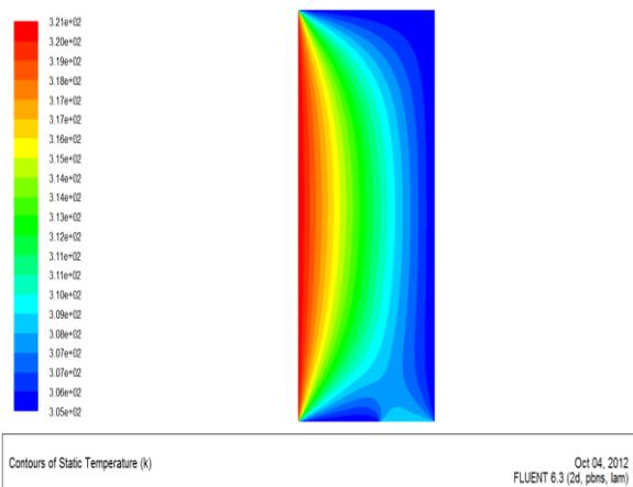
Fig. 17 Temperature Profile at  $q''=150 \text{ W/m}^2$  and  $S=-1.6$
