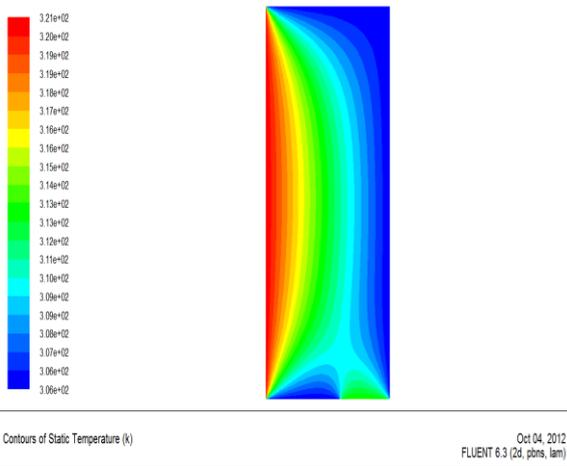
**Fig. 19** Temperature Profile at  $q''=150 \text{ W/m}^2$  and  $S=-5$
