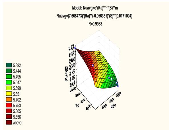
Fig. 12 Nusselt Number vs. Rayleigh Number and Stratification Parameter
