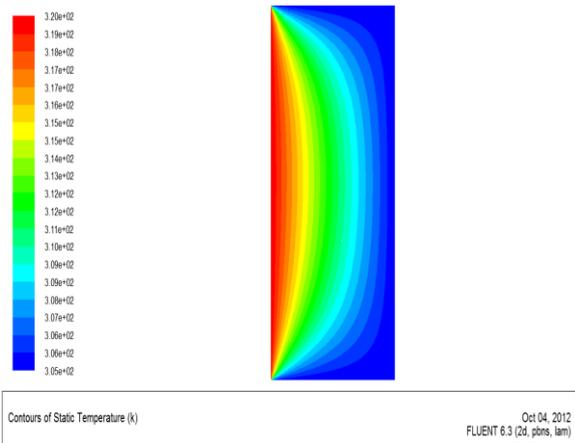
Fig. 15 Temperature Profile at  $q''=150 \text{ W/m}^2$  and  $S=0$
