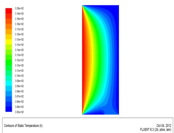
Fig. 16 Temperature Profile at  $q''=150 \text{ W/m}^2$  and  $S=-0.8$
