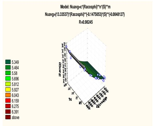
Fig. 14 Nusselt Number vs. Ra cosφ and Stratification Parameter
