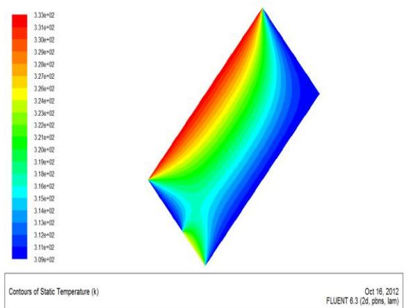
**Fig. 24** Temperature Profile at  $\phi=45^\circ$
