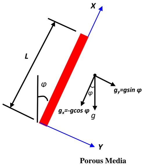
**Fig. 2 Geometry of the System**
