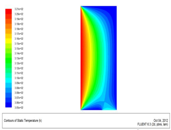
Fig. 18 Temperature Profile at  $q''=150 \text{ W/m}^2$  and  $S=-2$
