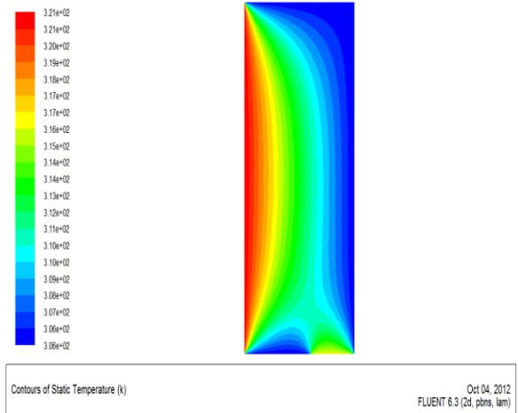
**Fig. 20** Temperature Profile at  $q''=150 \text{ W/m}^2$  and  $S=-10$
