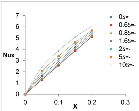
Fig. 7 Local Nusselt Number for  $q''=150 \text{ W/m}^2$  and  $\phi=0^\circ$
