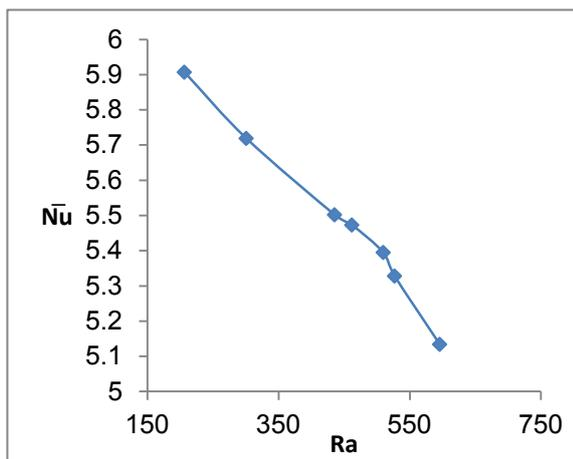
Fig. 11 Average Nusselt Number at  $q''=150 \text{ W/m}^2$  and  $\phi=0^\circ$
