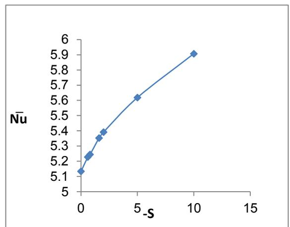
Fig. 10 Average Nusselt Number for  $q''=150 \text{ W/m}^2$  and  $\phi=0^\circ$
