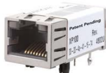
Figure 9: Embedded Web Server
