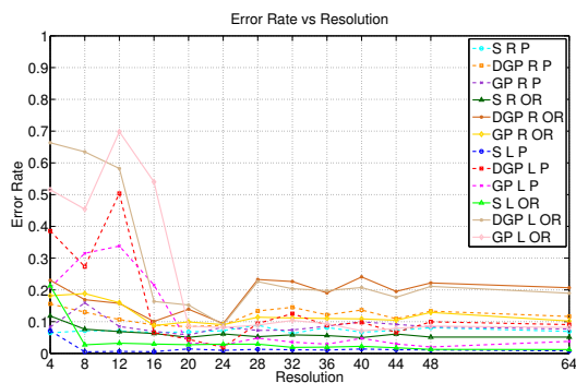
Fig. 5. The average error rate of various recognition algorithms as a function of the resolution of hand images using CPP pre-processing. Compare the trends of these plots with those of Figure 4, which only differ because of another pre-processing scheme implemented.
