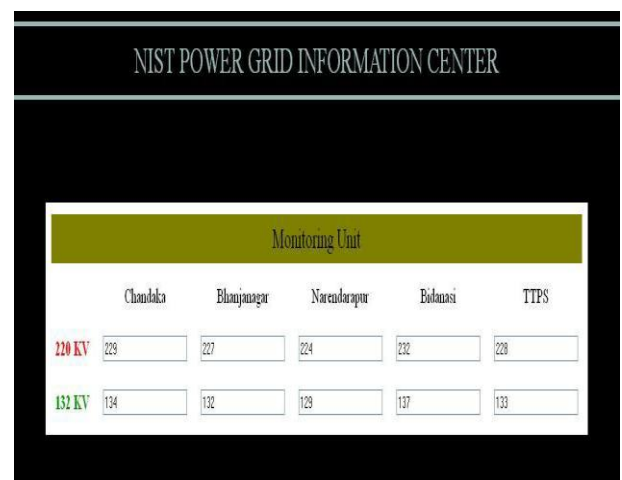
Figure 11. The monitored value of current bus bar voltage at different substation level.
