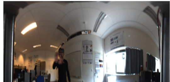
Fig. 5. Unwrapped image obtained by spherical transformation.
