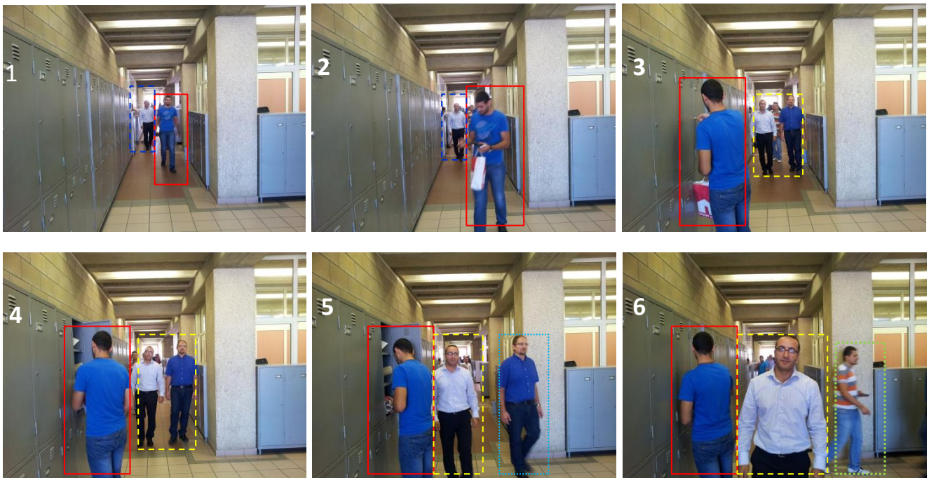
Fig. 5. Tracking of multiple subjects: The self-splitting PSO automatically generates new swarms to new or separating subjects in real-time.
