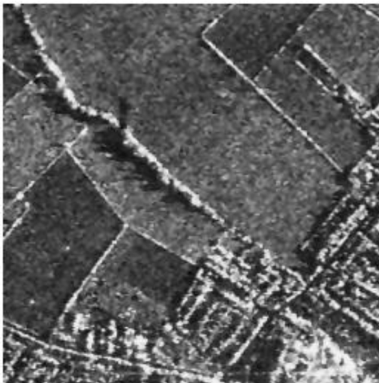
Figure.9 The de-speckled image using Frost filter
