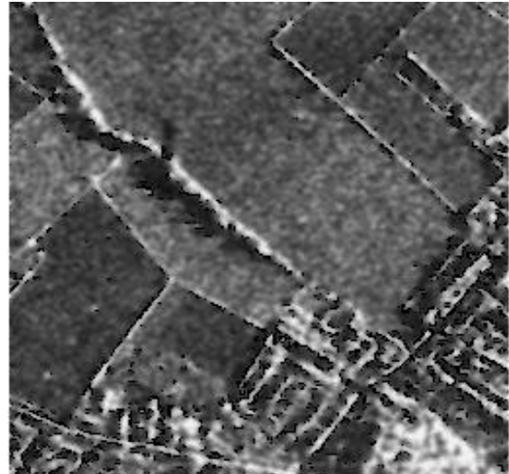
Figure.11. The de-speckled image using Gamma MAP filter
