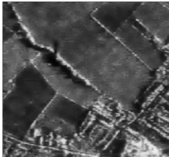
Figure.12 The de-speckled image using wavelet based scheme
