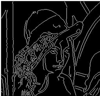
Figure 9.a) Lena after applying Canny
