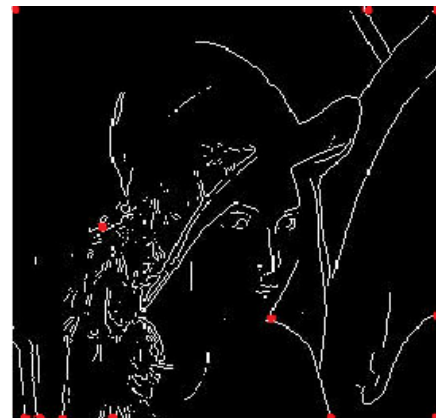
Figure 7.b) Harris corner implemented on Prewitt's edge detected image (Fig 7.a)
