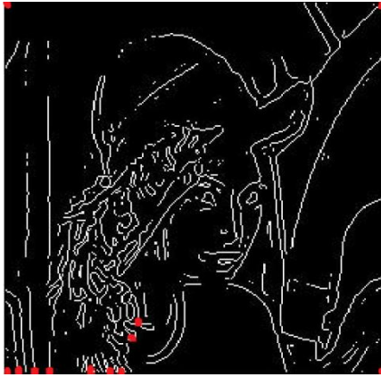
Figure 10.b) Harris corner implemented on Zerocross edge detected image (Fig 10.a)
