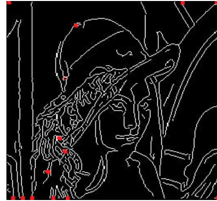
Figure 9.b) Harris corner implemented on Canny edge detected image (Fig 9.a)
