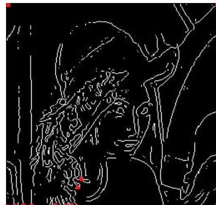
Figure 9.b) Harris corner implemented on LoG edge detected image (Fig 9.a)
