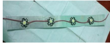
Fig 4: Back-side of the white LED panel showing series configuration.
