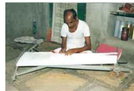
c) Marking of Design on Weft on Tie & Dye Frame with Charcoal/Fountain Pen Graphed design for tie-dyeing the threads before putting on loom.
