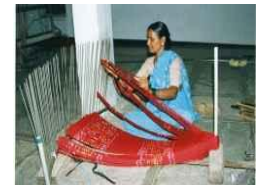
f) Placing of the Tie & Dye weft on Tie & Dye Frame for Rewinding
