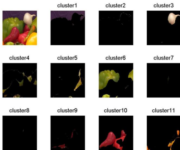
Figure 7: Onion and 16 clusters with window size 5, ( \sigma_d ) = 5, ( \sigma_r ) = 0.2, T=15, rest cluster are on second screen not displayed here.
