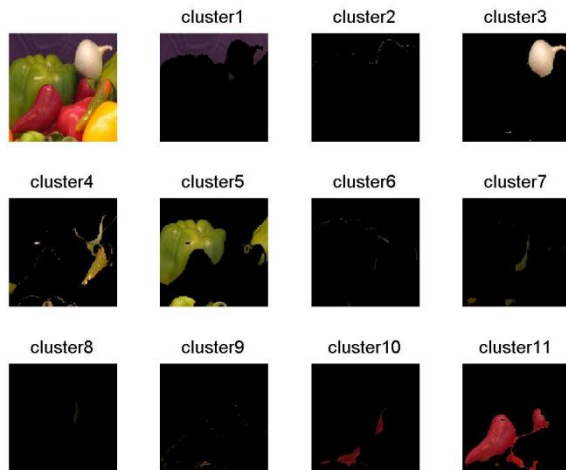
Figure 7: Onion and 16 clusters with window size 5, ( \sigma_d ) = 5, ( \sigma_r ) = 0.2, T=15, rest cluster are on second screen not displayed here.
